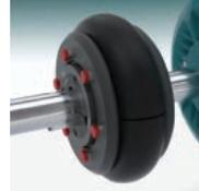
10. Tighten clamping ring screws alternately and evenly (half turn at a time), working round each flange until the required screw torque is achieved (Table 1).
