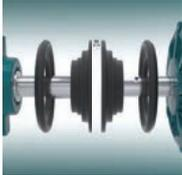
5. Bring shafts into line until dimension 'M' is obtained (Table 1). If shaft end float is to occur, locate the shafts at mid-position of end float when checking dimension 'M'. Note that shaft ends may project beyond the faces of the flanges if required in this event, allow space between shaft ends for end floats and misalignment.
