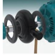
9. To ensure proper seating, it may be necessary to strike the outside diameter of the tyre with a small mallet. When seated there should be a gap between the ends of the tyre as shown in Table 2.
