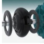
8. Open out tyre and fit over coupling flanges ensuring that the tyre beads seat properly on the flanges.
